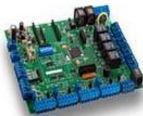
4 DOOR ACCESS CONTROL PANEL
